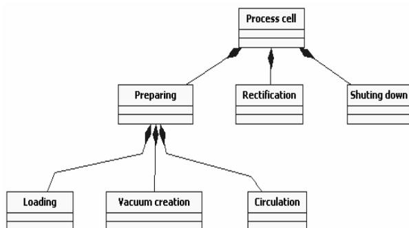
Fig.2: S88 hierarchy of the Industrial plant for Distillation of Sulphate Turpentine
