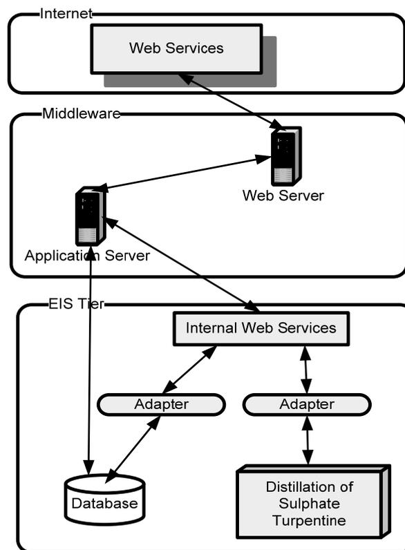
Fig.4: Web Service Architecture of Batch Process
