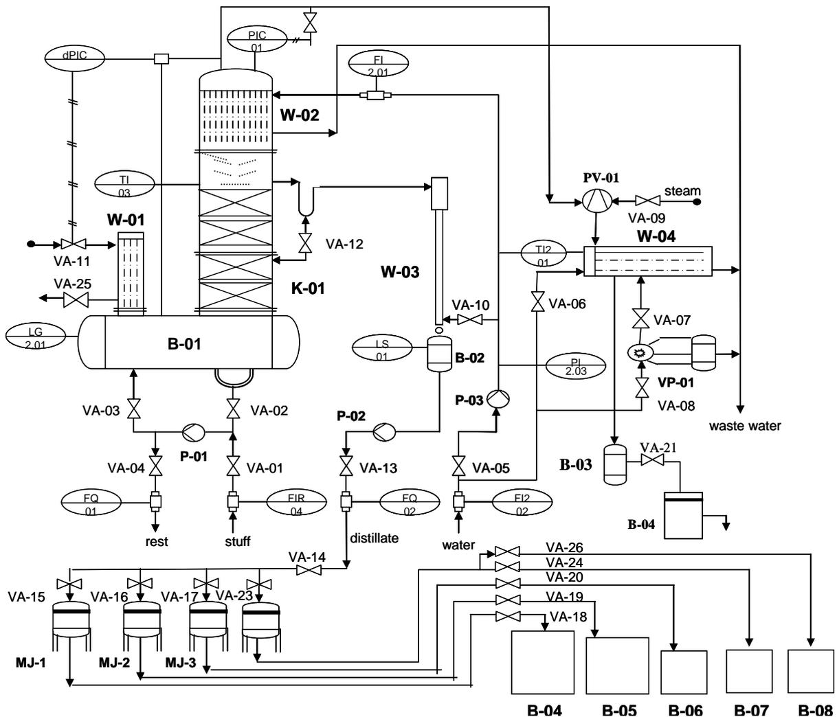
Fig.1: P&ID of the Industrial plant for Distillation of Sulphate Turpentine (UNIT according to S88 Batch Control Standard)
