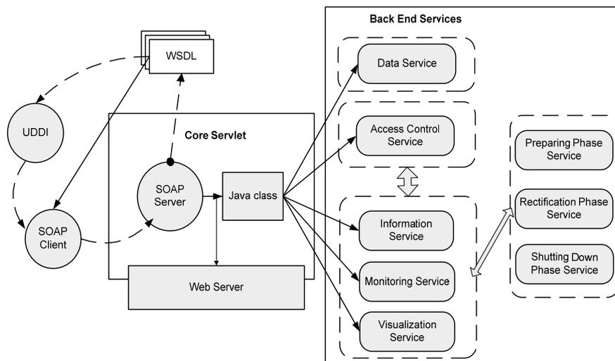
Fig.5: Web Service Architecture of Batch Process
